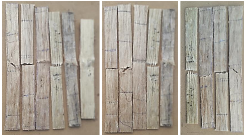
Figure 5:8 Specimen after Impact Test and Delamination failure
