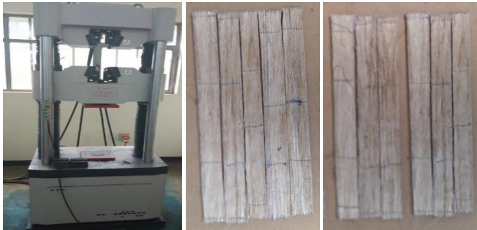
Figure 3:12 Compression testing machine and Specimen before test
