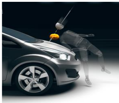
Figure 2:7 Head impact (Crash) testing of Car Bonnet at 40 km/h
