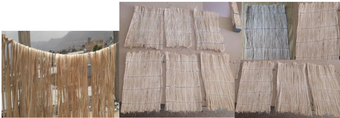
Figure 3:2 Extracted Fiber and Unidirectional Mat of Jute Fiber
