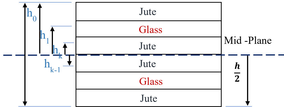
Figure 3:18: Laminate of the composite Plate plies via mid plane
