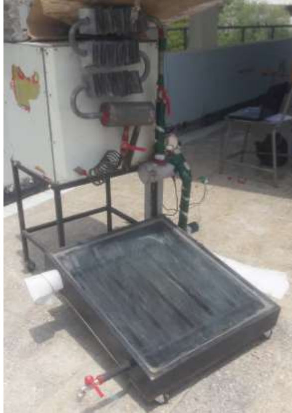
Figure 4. 15: The vapor absorption refrigeration system
