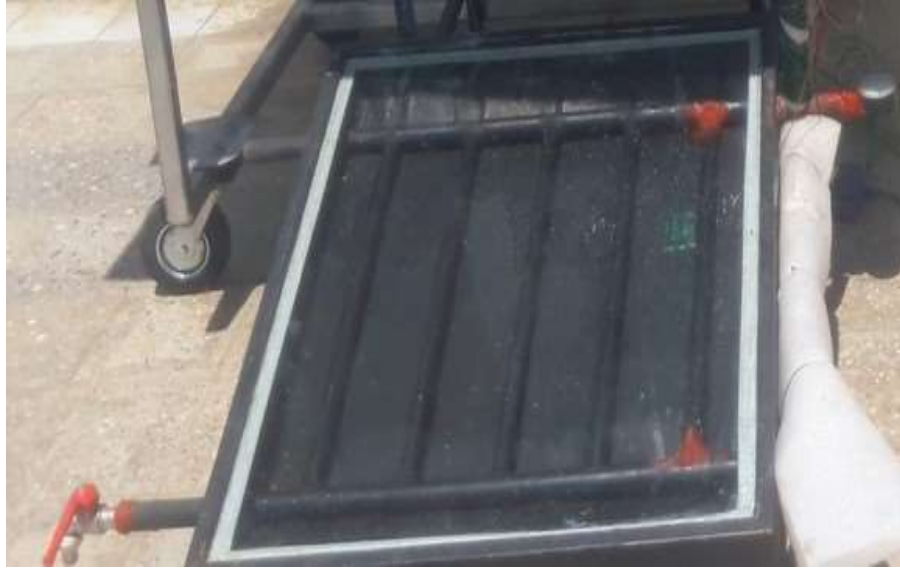
Figure 4. 4: Solar collector and generator
