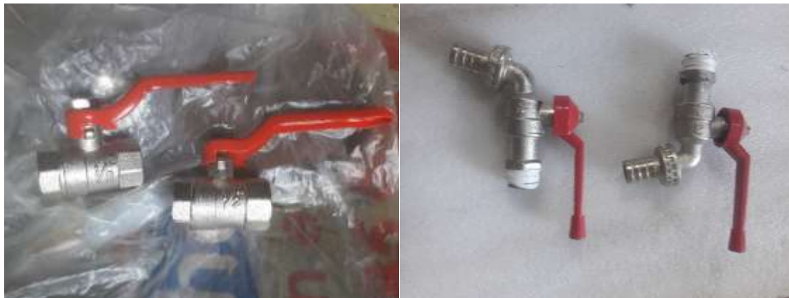
Figure 4. 11: Shutt off valves
