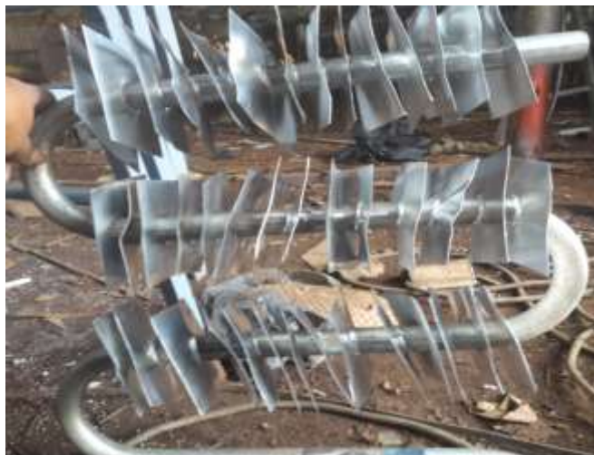
Figure 4. 5: Condenser with aluminum fin
