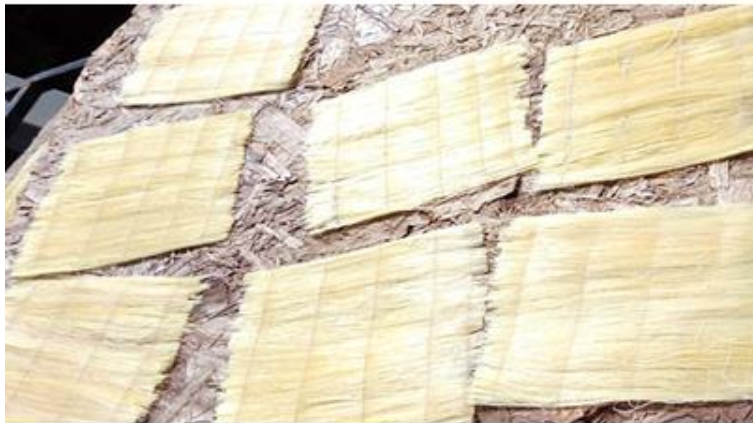
Figure 3-2: Unidirectional continuous sisal plies made by sewing.
