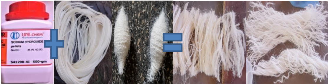
Figure 3.4 Sisal and wool fiber before and after treatments
