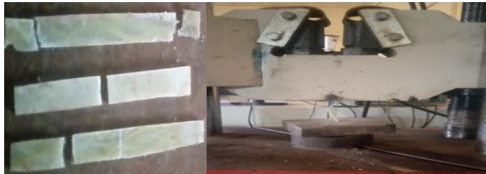
Figure 3.6 Compression test using a universal machine
