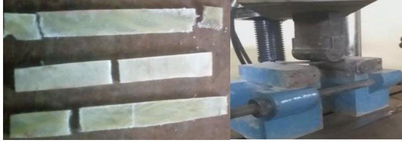
Figure 3.7 Flexural test using a universal machine
