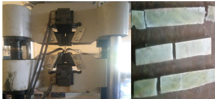
Figure 3.6 Tensile test using a universal machine
