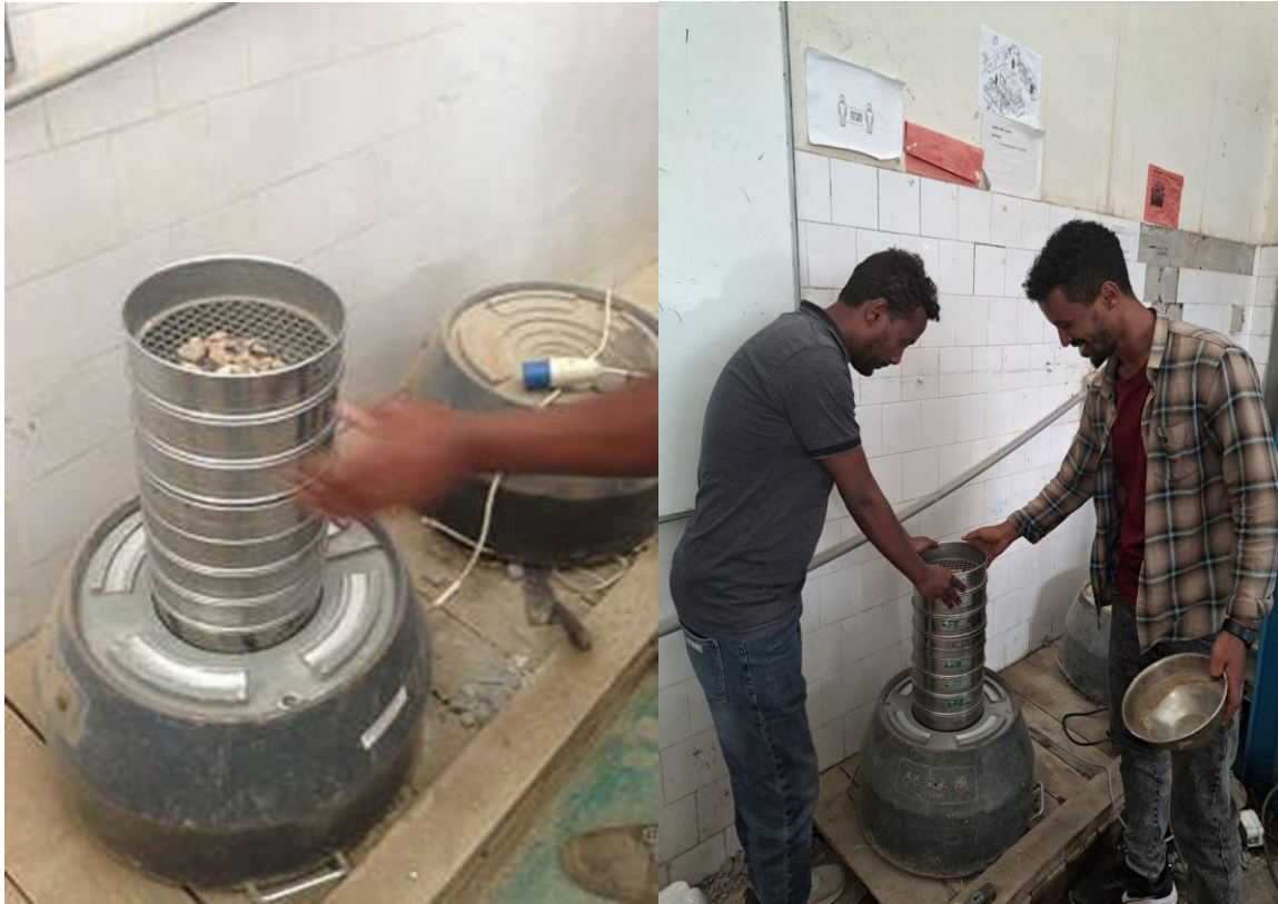
Figure 3-3 Set of sieves for fine aggregate
