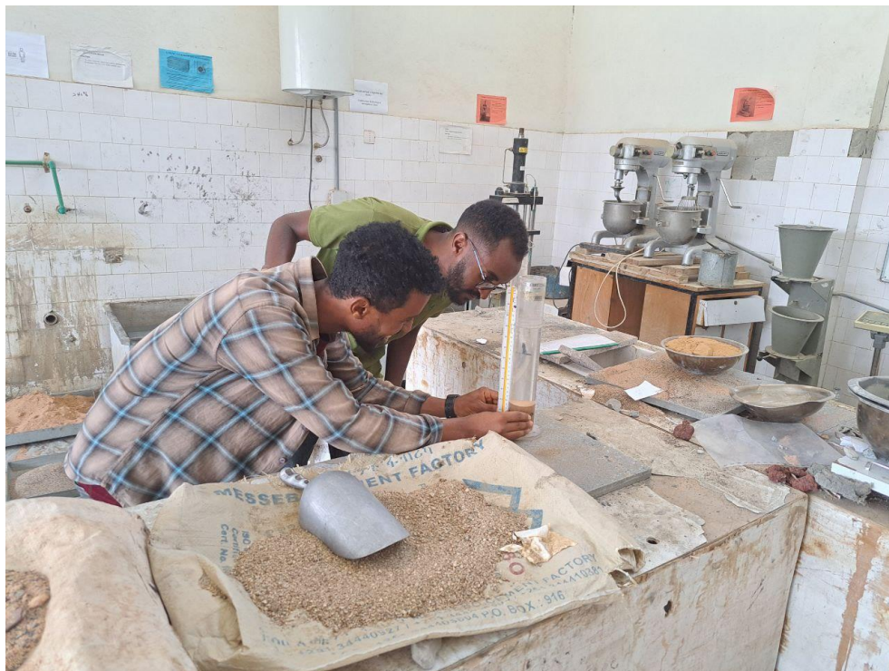
Figure 3-2 silt content test
