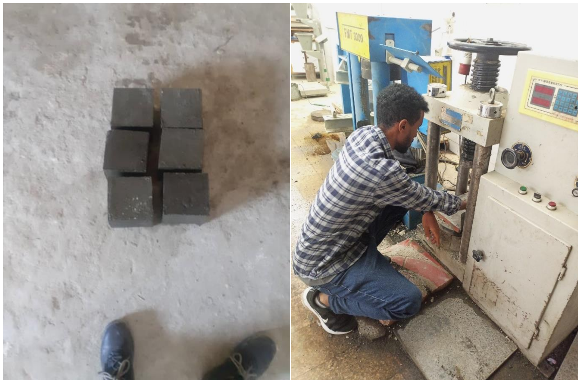
Figure 3-7 compressive strength test
