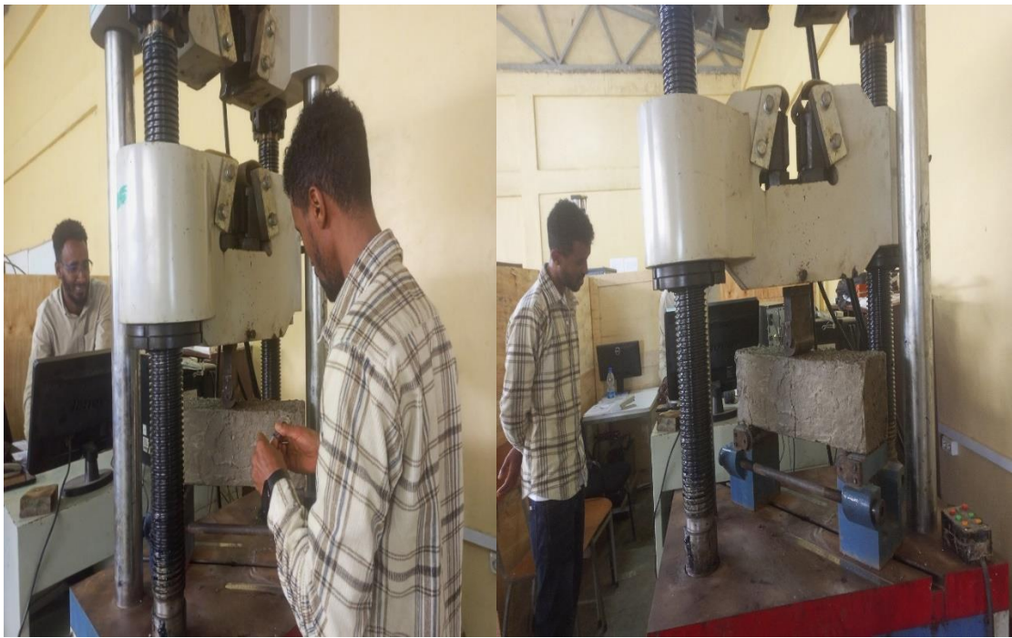
Figure 3-8 Compressive and flexural strength tests
