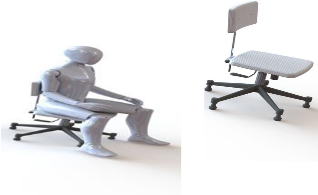
Figure 24 the proposed 3D Pneumatic Cylinder adjustable sewing operator chair design
