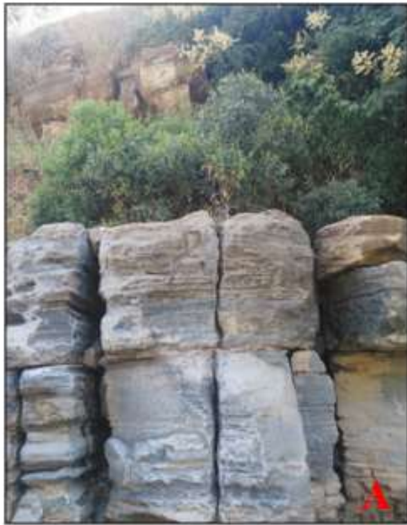
Figure 13: Field photographs of black limestone exposures in Mayalem quarry area.( A) Well-jointed black limestone blocks showing vertical to sub-vertical joints sets.(B) Outcrop illustrating bedded black limestone with visible stratification and joint planes.
