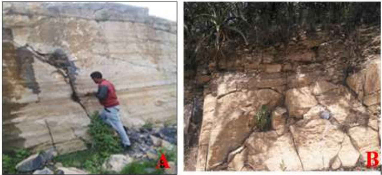
Figure 12: Field photographs of black limestone exposures in Kokolo quarry area :(A) Taking intact rock strength using Schmidt -hammer and the right image as (B) shale-limestone intercalations.
