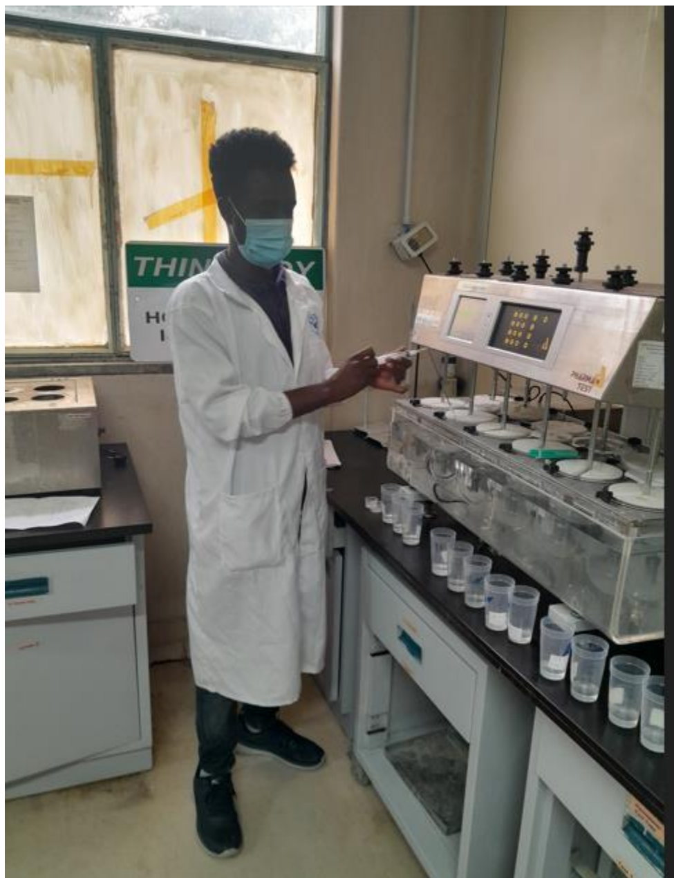
Annex 11: Image when performing Dissolution profile of different brands of Metformin tablets
