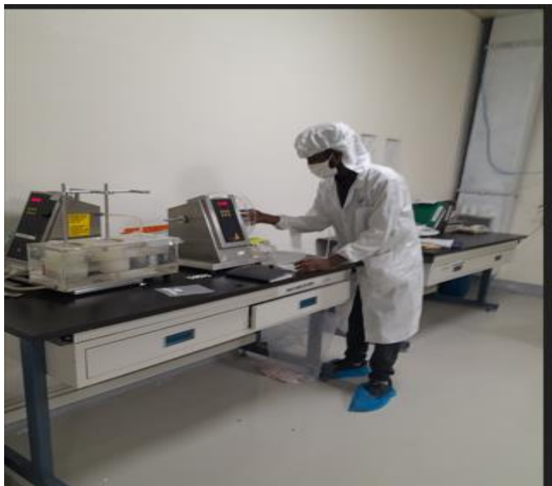
Image captured when performing Disintegration time and Friability Test in APF
