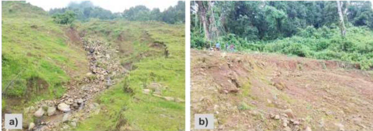
Figure 11: Representative unconsolidated deposits. (a) Alluvial sediments within a riverbed; (b) Colluvial materials along the backslope of a road.
