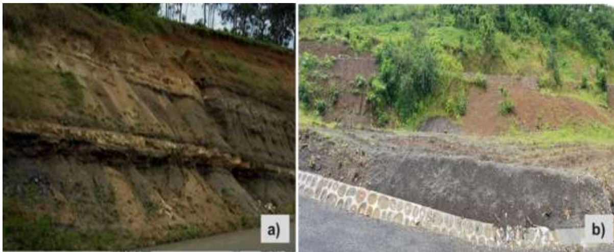
Figure 15: Representative lower trachyte flows. a) Km 31+960: Showing Lower Trachytes exposed around Felegeselam town with visible flow banding and distinct paleosol layers. b) Km 39+480: Highlighting the separation of lower trachyte by paleosol layers and surrounding vegetation.
