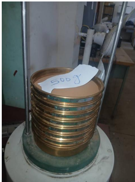
Figure 13 : Sieve analysis set up and process
