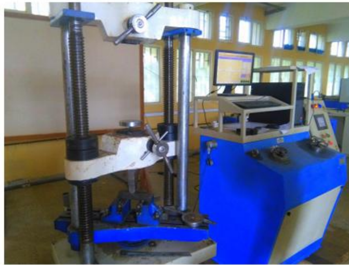
Figure 17 : Diagrammatic View of a Suitable Apparatus for Flexure Test
