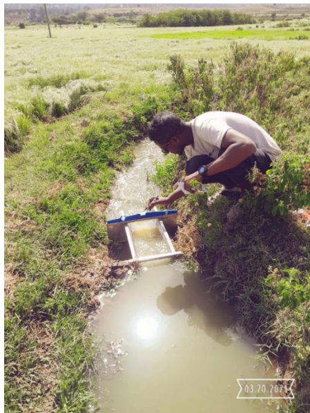
Figure 3b. Inflow-Outlet measurement using parshal flume
