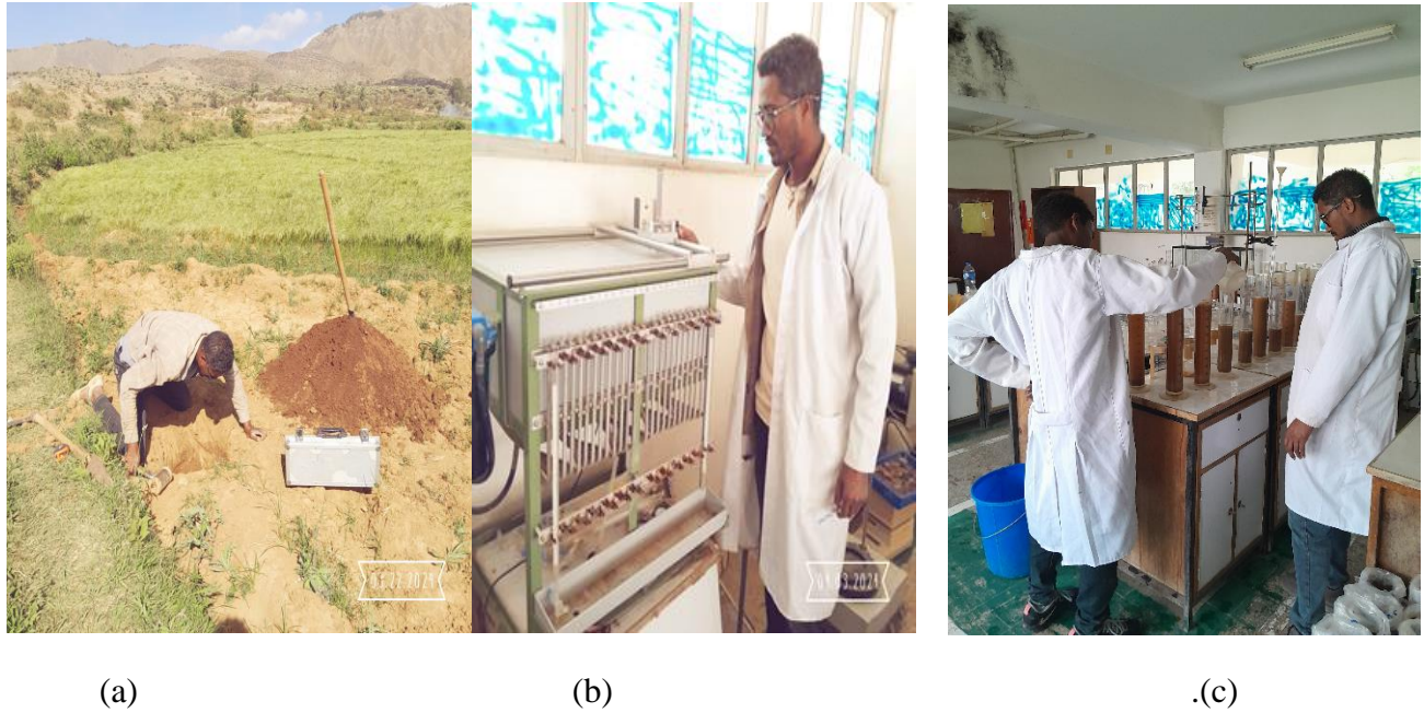
Figure 3a. (a) Soil sampling at the canal bank (b) constant-head perimeter (c) soil textural analysis using Hydrometer at Mekelle university soil laboratory service
