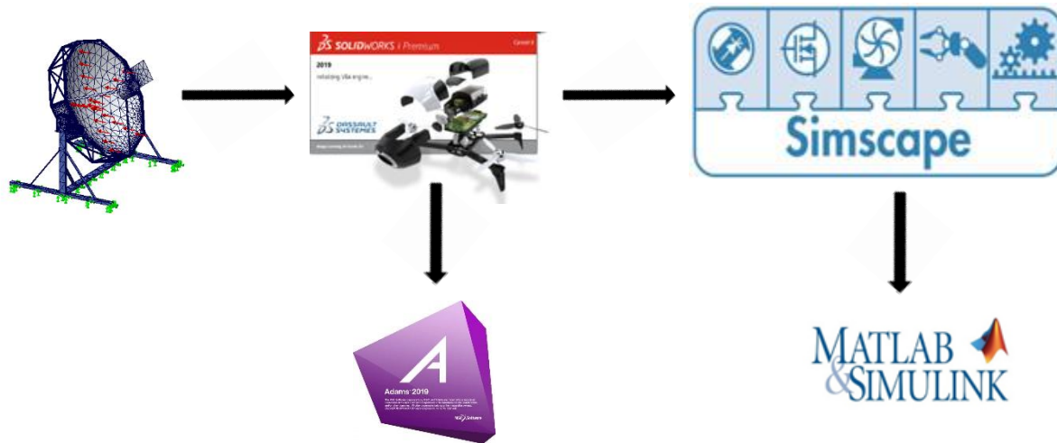
Figure 1.7: Software configuration used for the design, modeling and simulation of system
