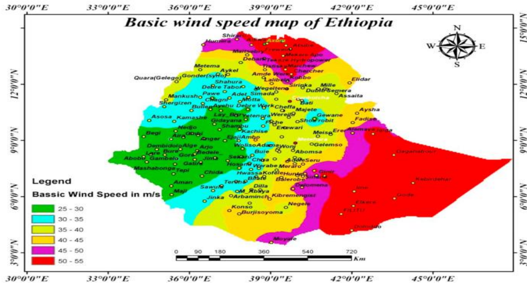
Figure 3.6: Basic Wind Speed map of Ethiopia [ Details of the weather stations and their locations, G. Melesse et al.]
