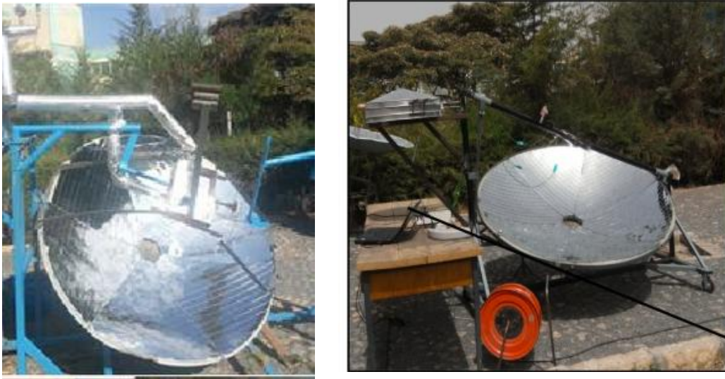
Figure 1.3: parabolic dish solar concentrators [14]
