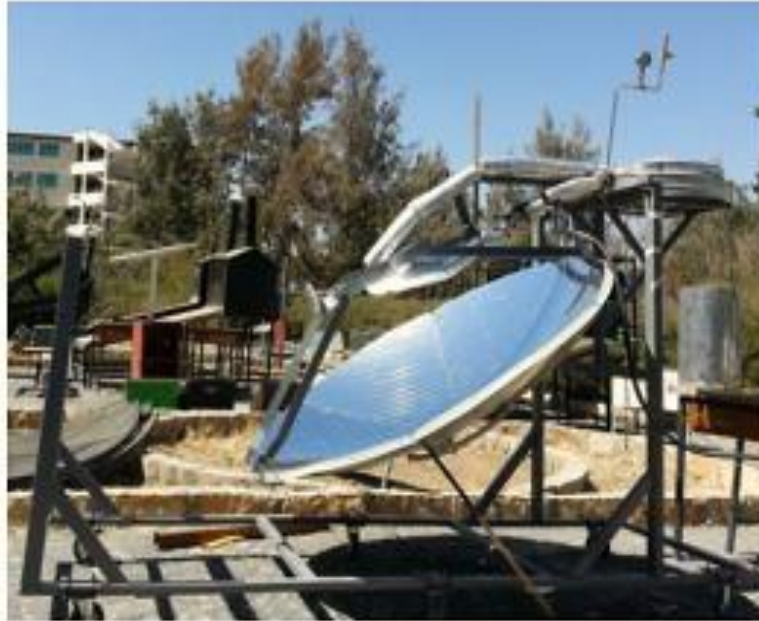
Figure 3.1: Existing parabolic solar concentrator [A. H. Tesfay, M. B. Kahsay, and O. J. Nydal, figure3]
