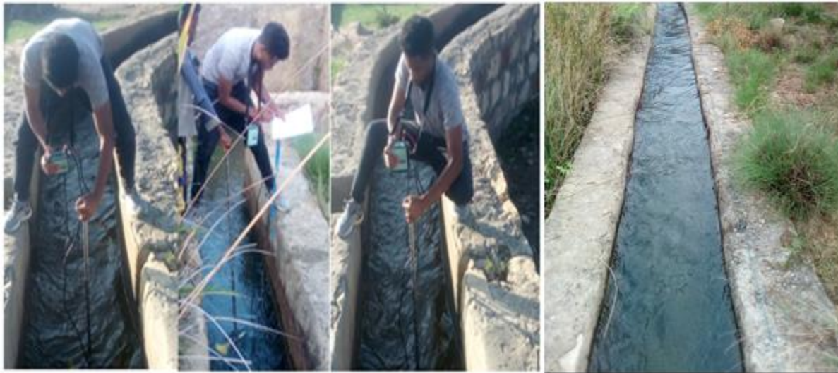
Figure 3-3: Flow measurement using current meter
