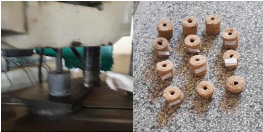
Figure 3.4: Production of the briquette using hallow cylindrical mold and computer controlled universal test machine and produced briquettes
