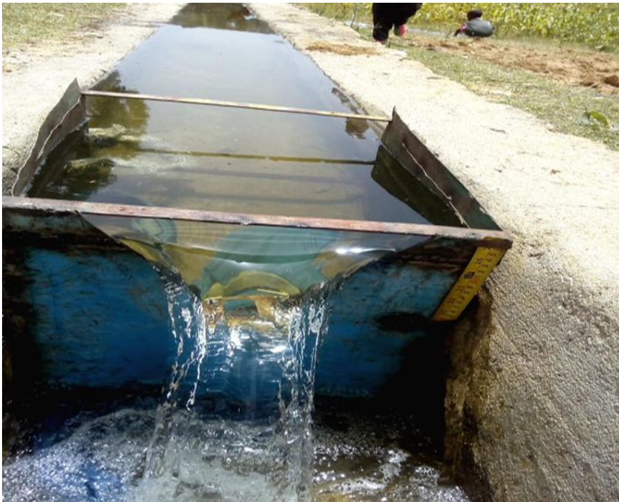
Figure 3. 8 Discharge measuring using V-notch weir in April
