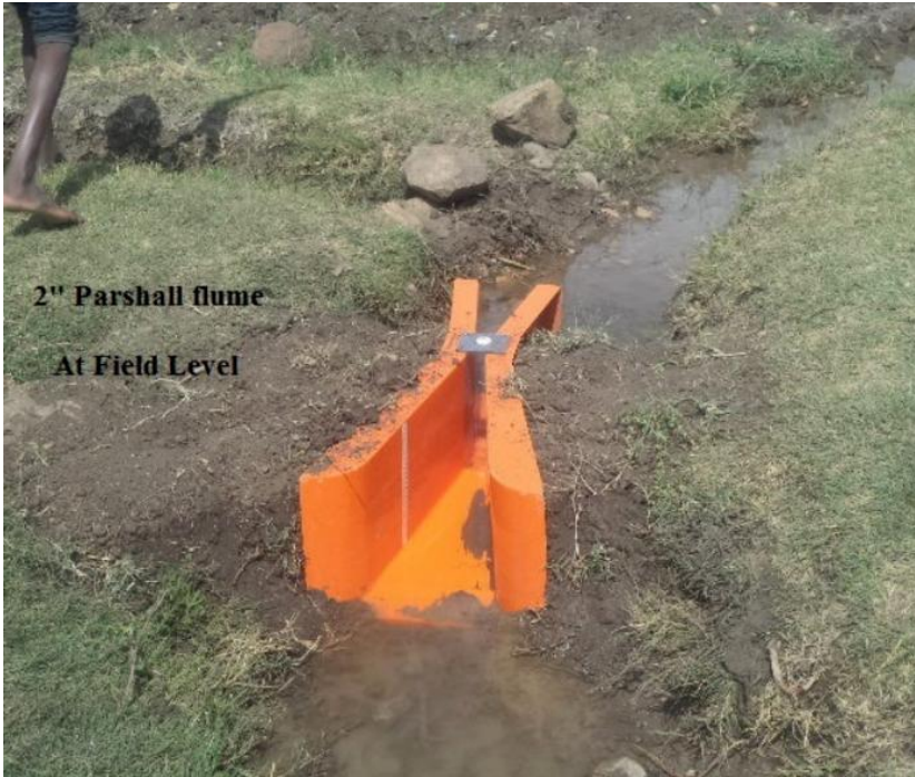
Figure 3. 9 Discharge measuring using 2” Parshall flume at farm
