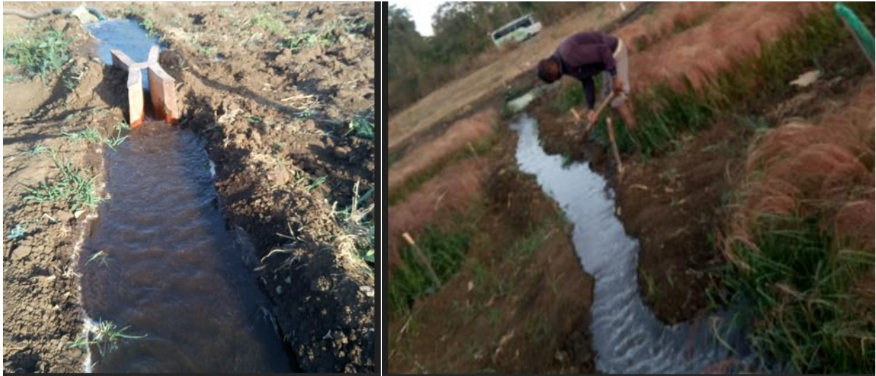
Figure 3: Two inch partial flume using for measuring flow discharge
