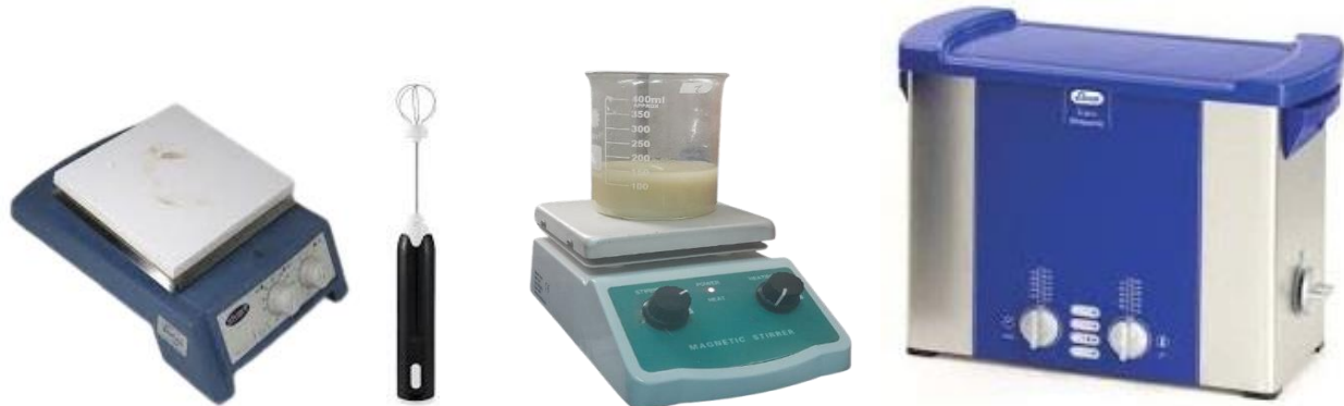
a) heat plate b) mechanical stirrer c) magnetic stirrer d) bath sonicator
