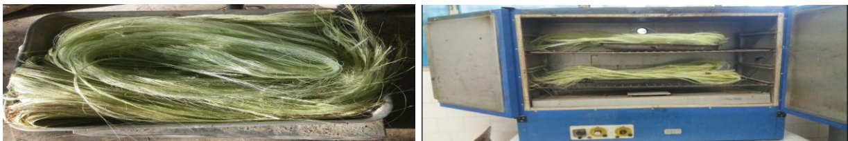
Figure 0.1.2: The treated sisal fiber dried in an oven at 60°C
