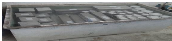
Figure 3.7: The curing specimens for 28 days
