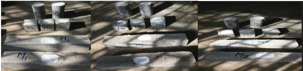
Figure 3.6: Figure of cube casting test
