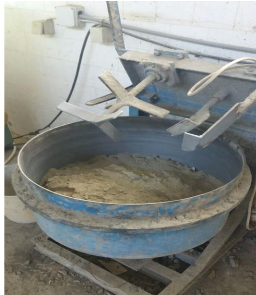
Photo: Mechanical mixer
