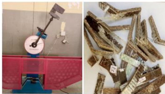
Figure 3-13: Charpy impact testing machine and Failure mode of specimens
