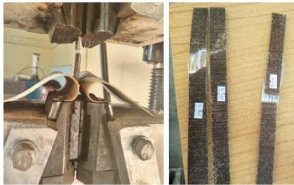
Figure 3-12: Tensile testing using universal testing machine and Failure mode of specimens
