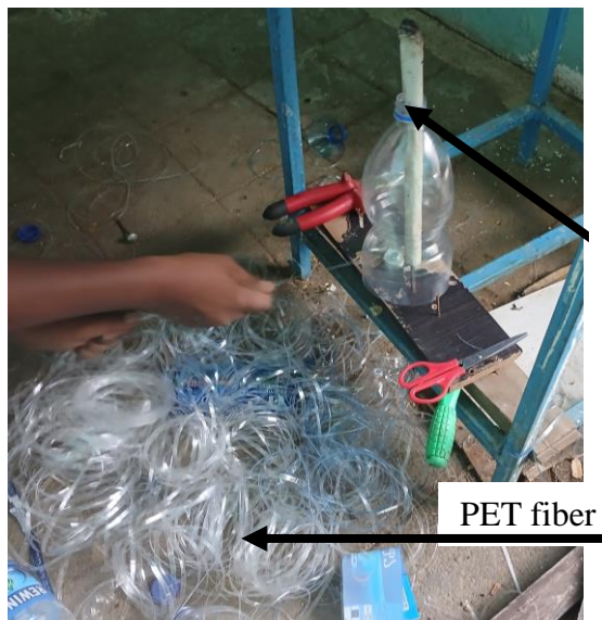
Figure 3-5: Plastic bottle cutting mechanism
