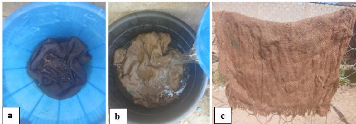
Figure 3-7: (a) jute immersed in the alkali solution and soaked (b) washed by pure water (c) fiber dried
