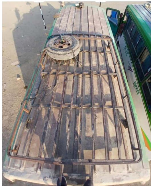
Figure 1-2: Roof of modified ISUZU NPR71 4570cc buses
